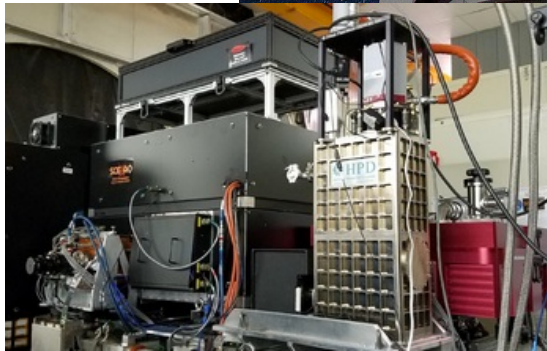
SExAO: extreme adaptive optics CHARIS: Integral Field Unit (IFU) Spectrograph
