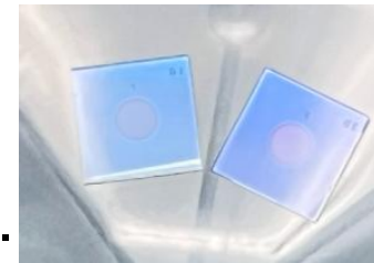
Example of phase masks for coronagraph (Photo. of previous version) and a vacuum testbed under development (Nishikawa+).
